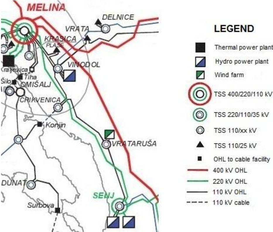
Figure 2. The transmission grid layout around WF Vrataruša
