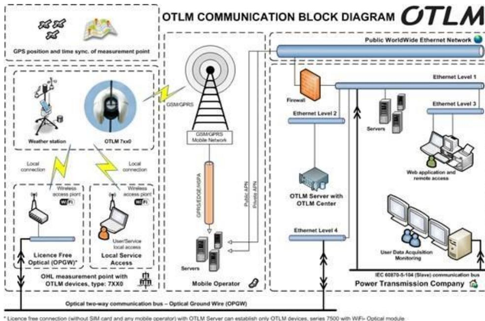
Figure 5. OTLM communication block diagram
