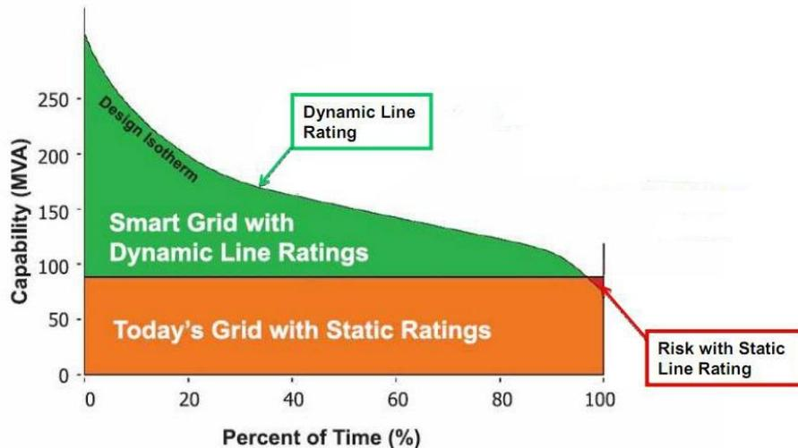
Figure 1. The relationship between static and dynamic line rating
