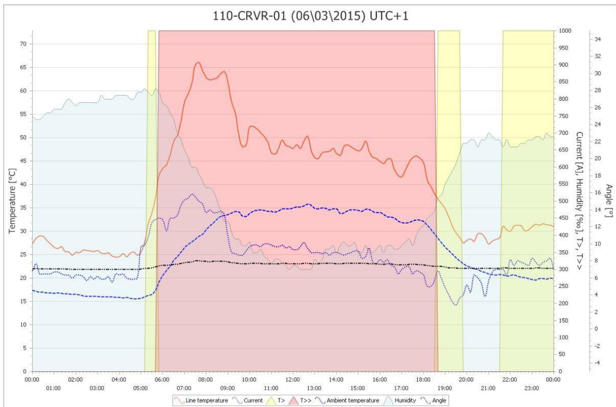
**Figure 8. The data received from OTLM device on 3.6.2015.**
