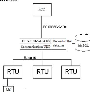
Figure 3: Protocol RTU <-> concentrator
